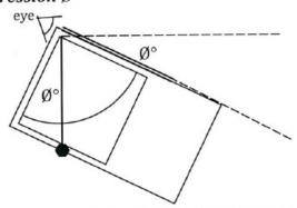
As the angle measurer is pointed downwards to the landmark the angle of depression can be read.
