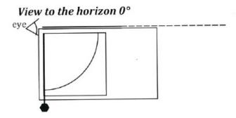
When the top of the angle measurer points to the horizon the angle will read 0°
